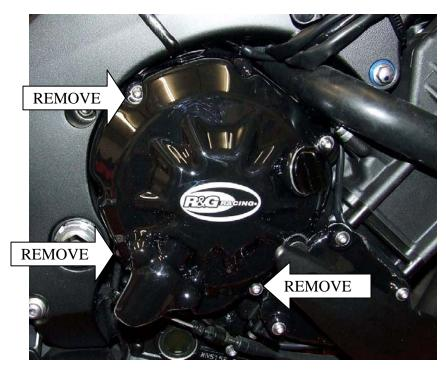
In this kit there should be 1 x Engine Case Cover 3 x M6 button head bolt 3 x M6 washers 3 x Black spacers 1 x 25mm length of heat shrink
