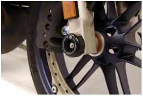
Please note that the way the kit is packed does not necessarily represent the way of mounting to the bike Please note that in cases where kits are packed with rubber washers holding the components onto the bolt – *the rubber washers should be thrown away*!
