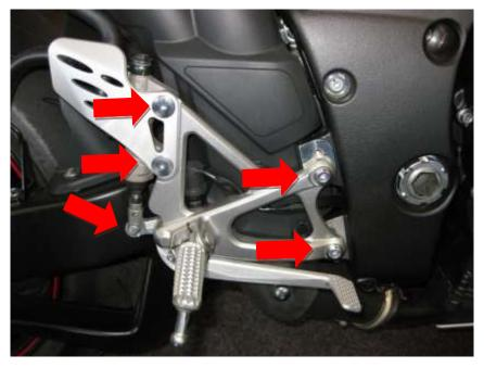
Connect the brake cylinder with the R&G brake cylinder adapter, find the right position for the Rearsets and connect them with the frame.
