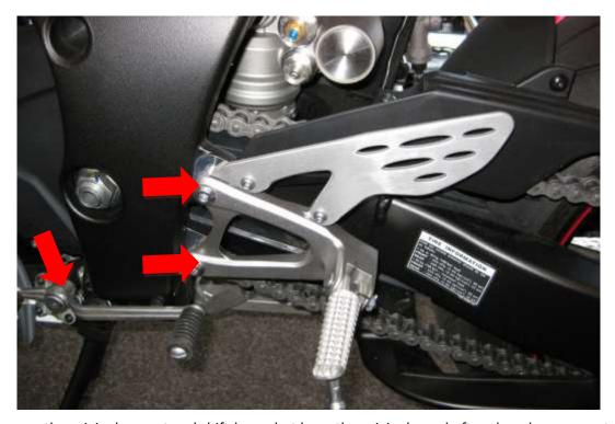
Remove the original rearset and shift-lever, but keep the original gearshaft and gearbox-connector.
