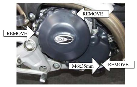
In this kit there should be: 1 x Engine Case Cover (ECC0046) 2 x M6x90mm long button head bolts 1 x M6x35mm long button head bolt
