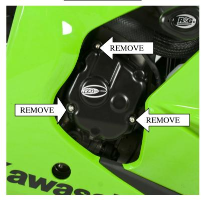
In this kit there should be: 1 x Engine Case Cover (ECC0096) 3 x M6x35mm long button head bolt
