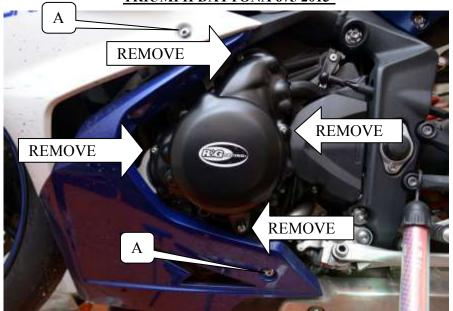
In this kit there should be: 1 x Engine Case Cover (ECC0141) 4 x M6x35mm long button head bolts
