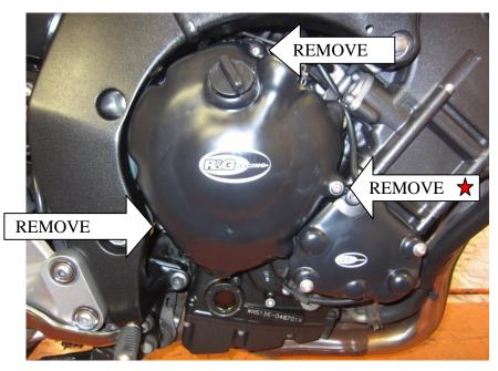
In this kit there should be: 1x Engine Case Cover (ECC0054) 3x M6 x 50mm long button head bolts 1x M6 Washer
