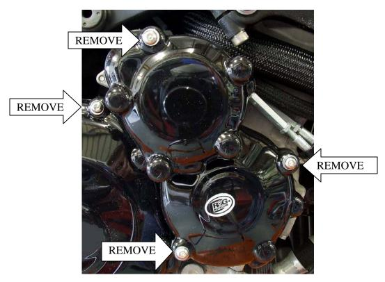
In this kit there should be: 1 x Engine Case Cover 4 x M6 button head bolts 4 x M6 washers 4 x black spacers 1 x 25mm length of heat shrink
