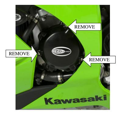
In this kit there should be: 1 x Engine Case Cover (ECC0094) 3 x M6x40mm long button head bolt
