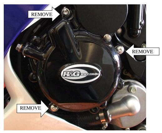
In this kit there should be: 1 x Engine Case Cover 3 x M6 button head bolts 3 x M6 washers 3 x Black spacers 1 x 25mm length of heat shrink
