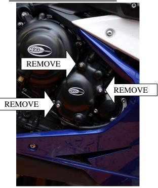
In this kit there should be: 1 x Engine Case Cover (ECC0142) 3 x M6x35mm long button head bolts
