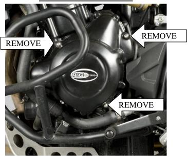
In this kit there should be: 1 x Engine Case Cover (ECC0106) 3 x M6x35mm long button head bolts
