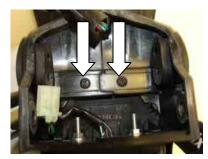
• Separate 2 halves of OEM tail bracket and under-tray by disengaging fastening clips and pulling apart (side-ways). This will allow you to remove wiring loom (keep for fitting to new licence plate holder-under tray).
