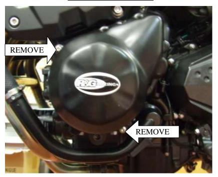
In this kit there should be: 1 x Engine Case Cover (ECC0074) 2 x M6x40mm long button head bolt
