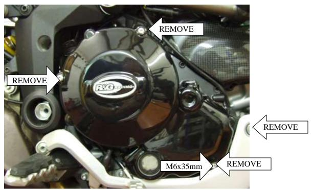
In this kit there should be: 1 x Engine Case Cover (ECC0082) 2 x M6x90mm long button head bolts 1 x M6x35mm long button head bolt
